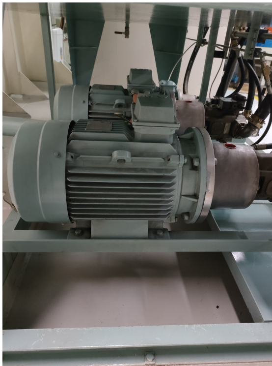
Figure 75: Hydraulic Pump For RoRo No1
