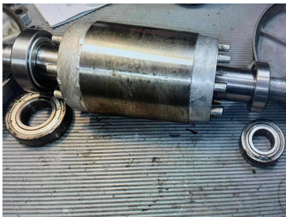
(a) Rotor Of CO2 Compressor
