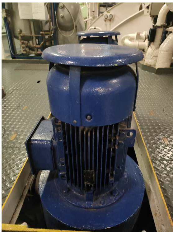
Figure 93: Main Engine Fresh Water Cooling(Jacket)
