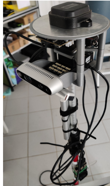
FIGURE 6.3: Placing of the RPi4 and the power bank in the initial mount of the components of the system.
