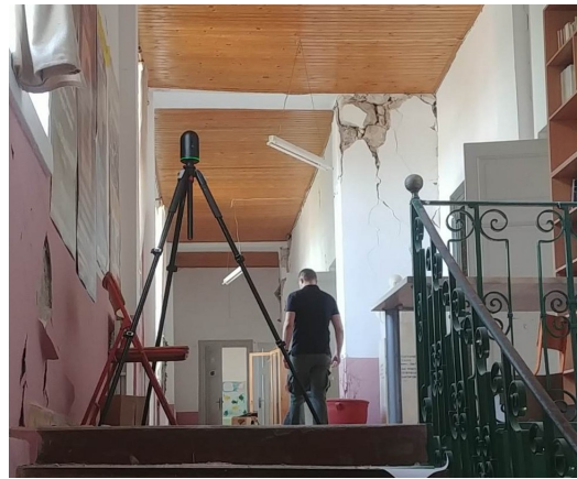
FIGURE 2.3: 3D Laser Scanner in a decommissioned school due to earthquake damage.
