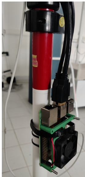
FIGURE 6.3: Placing of the RPi4 and the power bank in the initial mount of the components of the system.
