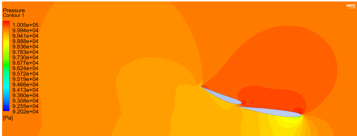
Figure 6.7 Static pressure distribution around the front wing, at the symmetry plane.
