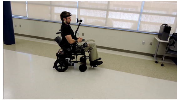
Figure 4: BCI Control of a Motorized Wheelchair for Disabled Individuals using a calibrationless SSVEP system https://www.youtube.com/watch?v=qhK572LJhSc
