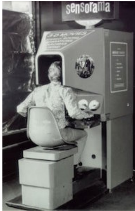
Figure 12: The Sensorama VR machine
