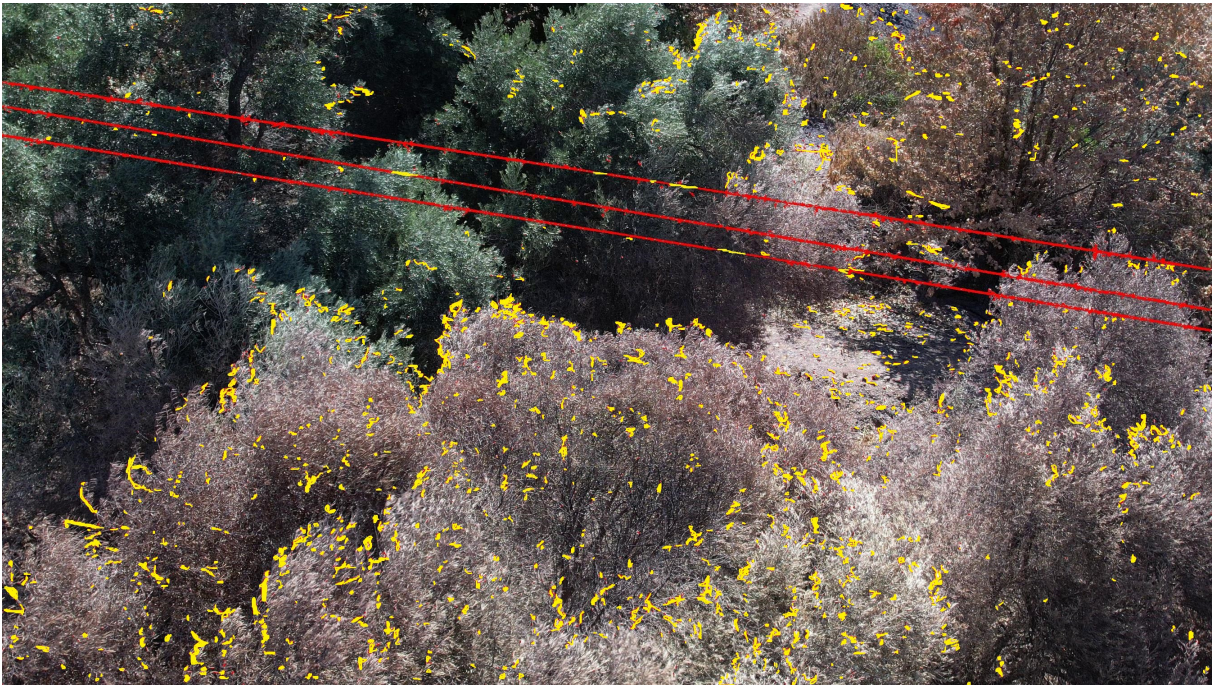
Figure 4.6: Segmentation Result of UNet. Detected lines are highlighted in red, while gaps and noise are highlighted in yellow.
