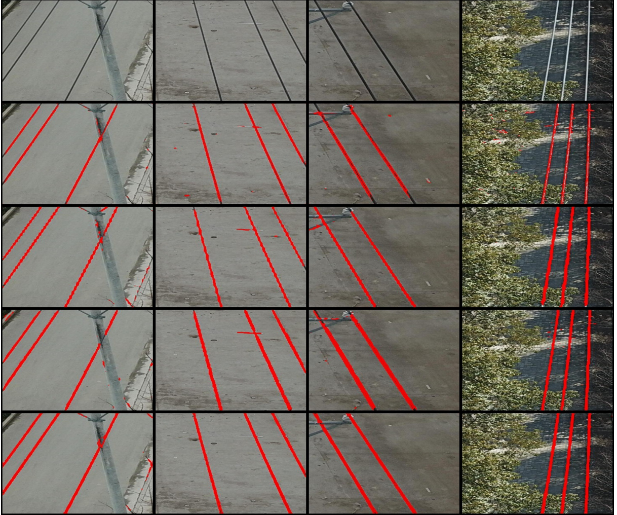
Figure 4.1: Visualizing PLDU: Segmentation Insights with 4 Deep Learning Networks. From Top to Bottom: Original Images, UNet Segmentation, Modified FCN Segmentation, DeepLab Segmentation, DLinkNet Segmentation.
