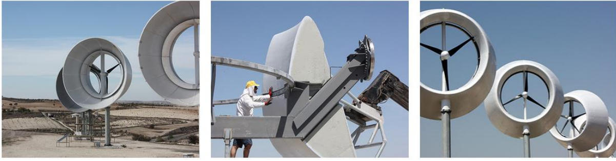
Figure 1.3: The full-scale prototypes of Hummingbird H15 DAWT model designed by OGT Greentech Ltd, with a rated capacity of 15 kW [Source: https://www.omnilinkgreentech.com ].
