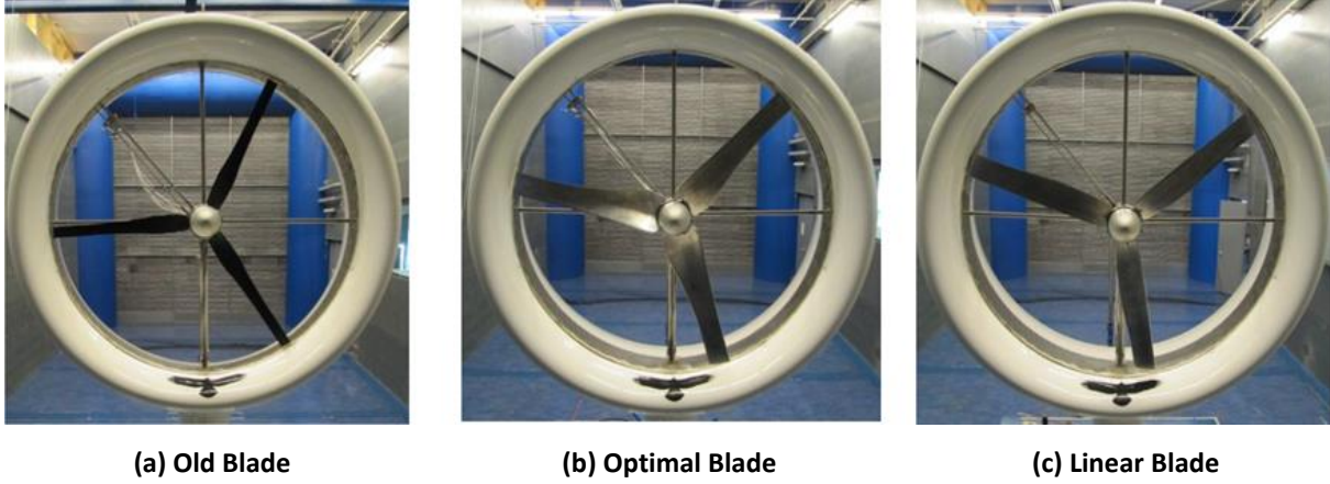
Figure 3.8: The three blade designs of Donqi Urban Windmill (van Dorst, 2011).
