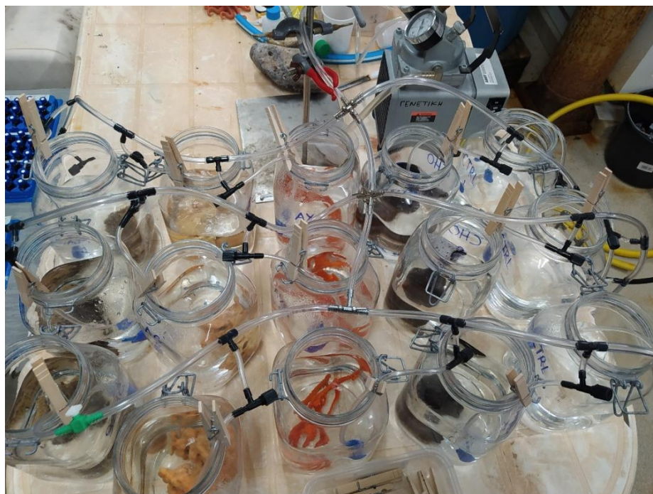
Figure 4.1. The experimental set-up established for the in vitro investigation of sponges bioremediation capacity against aquaculture-related dissolved organic pollutants.
