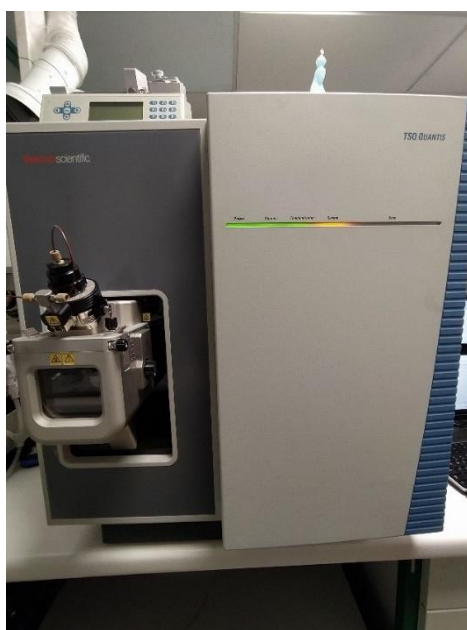
Figure 5.2. The LC-MS/MS equipment used for dereplication of farmed and wild sponge extracts at NOVA University of Lisbon, Portugal.
