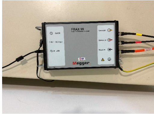
Figure 4.7: FRAX front panel with input connections
