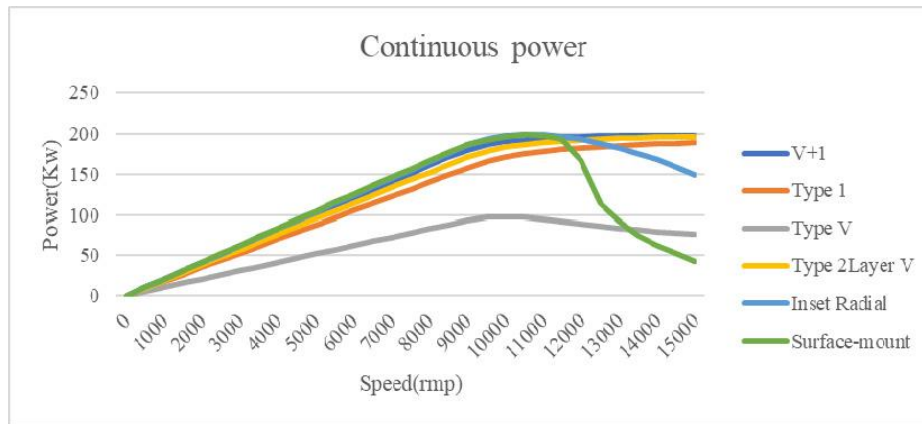
Figure 1.16: Power-Speed characteristic of PM structures [3]
