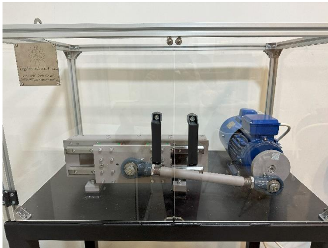
Figure 5.39: The developed device for mechanical stressing of the poles
