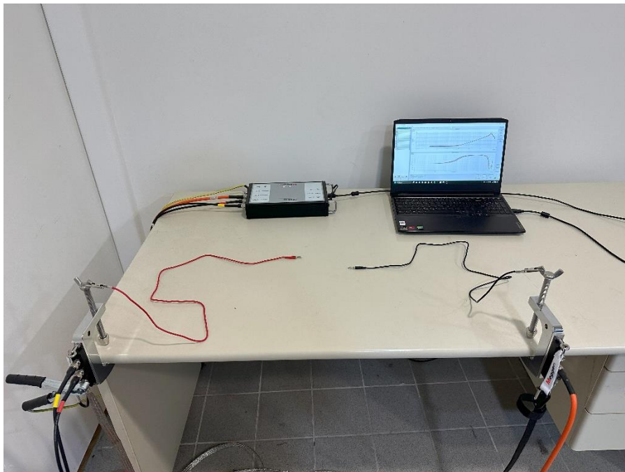
Fig6.1: Impedance Spectroscopy Set-Up
