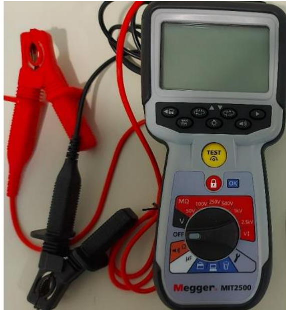
Fig.6.3: Portable Megger Device
