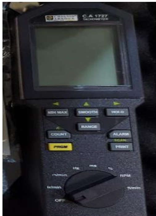
Fig.6.4: Digital Tachometer
