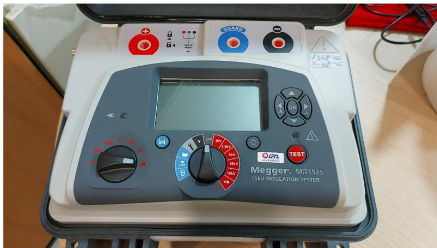
Fig6.2: Megohmmeter 15kV Insulation Tester
