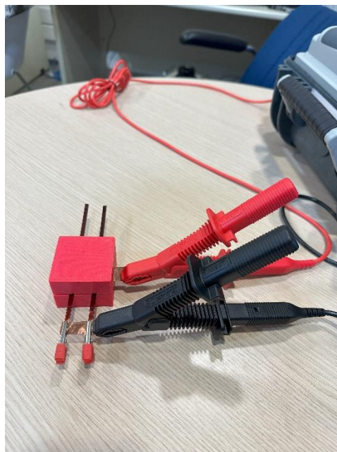
Fig. 6.8. Setup for the measurement of the turn-to-turn insulation resistance.
