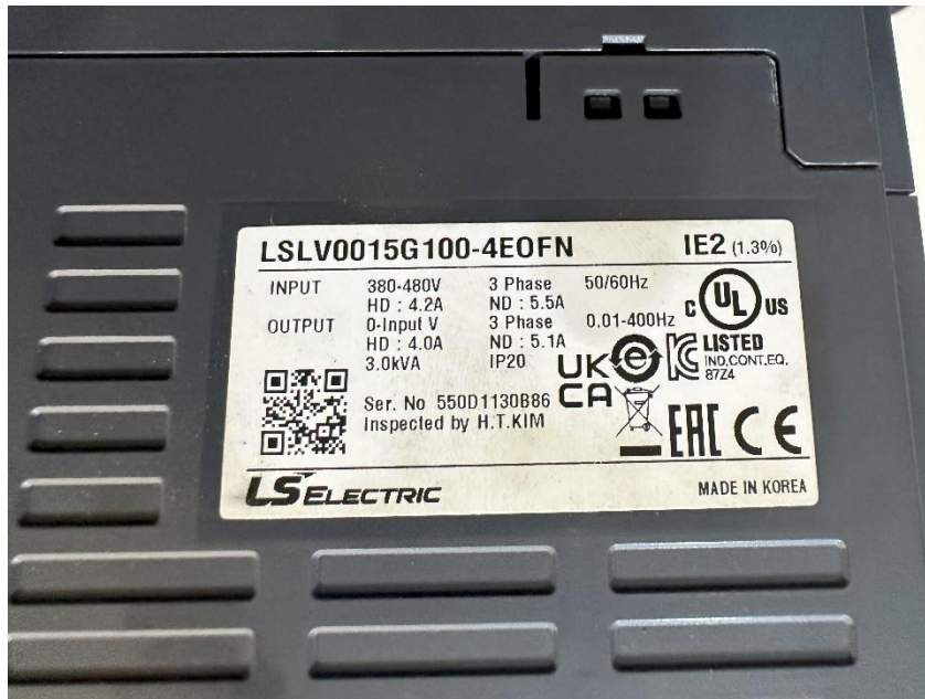
Fig.6.11: Inverter used for the mechanical stressing machine drive
