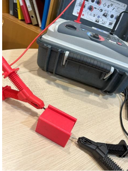
Fig.6.7: Setup for measuring the coil-to-pole insulation resistance.
