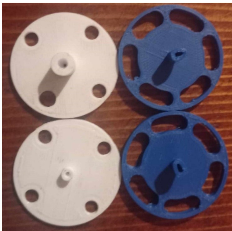
Figure 6-2: Nozzles produced via FDM 3D-printing.
