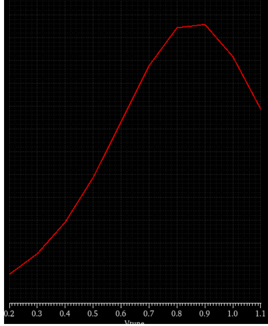
Figure 40: Representation of KVCO vs. V_{\text{tune}} , with 0.3V V_{\text{gate}} ( \Delta C / \Delta V_{\text{tune}} ).
