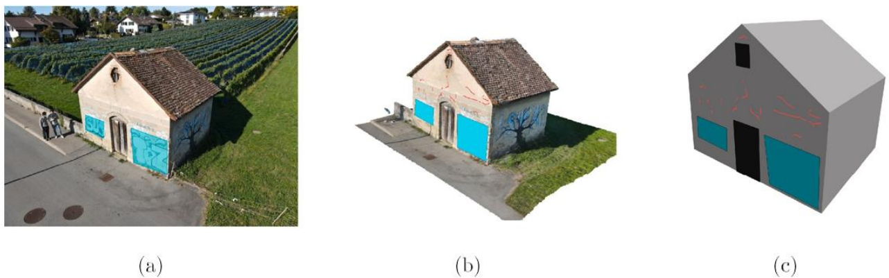
Figure 10: Augmenting models with extra semantic information. (a) Semantic information segmented from images. (b) MVS textured model, cracks and extra semantic information. (c) DADT composed of LOD3, cracks and extra semantic information.
