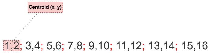
Figure 28: String representation of a trajectory
