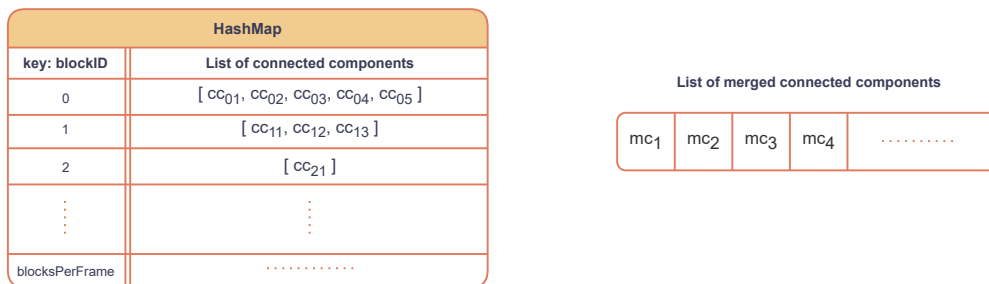
Figure 25: The necessary data structures for the implementation of the connected component algorithm
