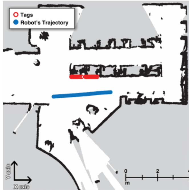
Figure 2.10: Campaign IV: Real map of the library produced by the Cartographer algorithm, including the robot's estimated trajectory and the actual location of the tags.
