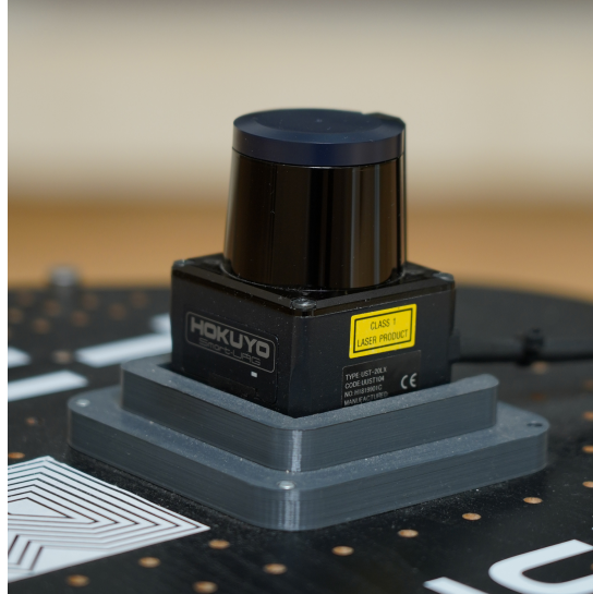
Figure 1.2: Hokuyo UST-20LX mounted on Turtlebot.
