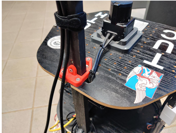
Figure 1.8: The 3D printed pole mounting adapter (red).
