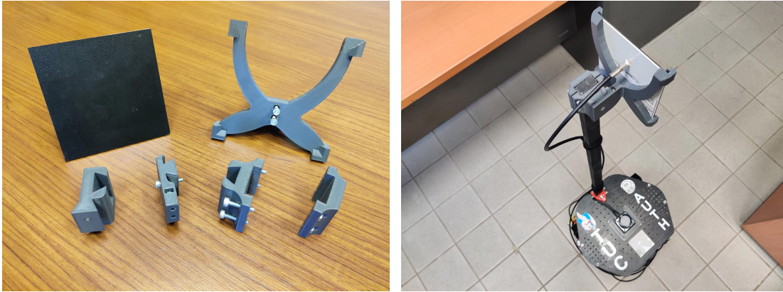
(a) Antenna holder, adapter and mounting bracket. (b) The whole assembly mounted on the robot.
