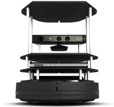
Figure 1.1: The default configuration of the Turtlebot2 platform.
