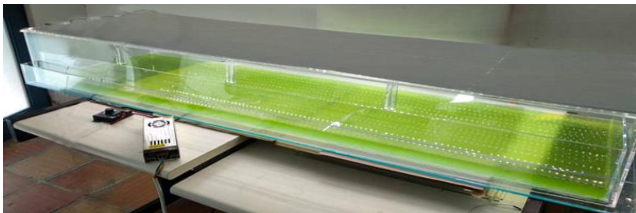
Figure 44. Photograph of the pilot-scale flat-panel photobioreactor that was used in the cultivation experiments of EMS1 Stichococcus sp.
