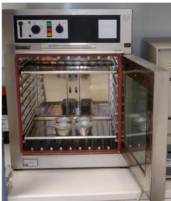
Figure 58. Laboratory hot air oven used for microalgae biomass convective drying.
