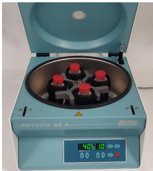
Figure 54. Centrifuge device used to separate the microalgal biomass from the culture medium.
