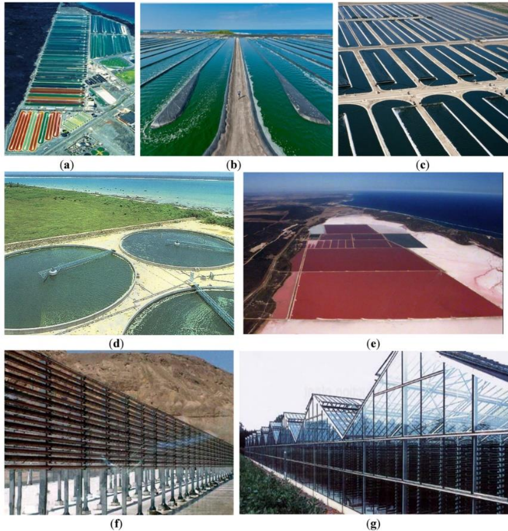
Figure 9. Commercial microalgae production systems: ponds and photobioreactors. (a–c) Commercial production systems using paddle wheel mixed raceway pond systems. (d) , circular ponds, each \sim 500 \text{ m}^2 , with central pivot mixing; (e) unmixed ponds (f–g) tubular photobioreactors (Benemann, 2013).
