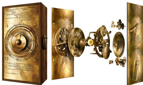
Figure 1.1: An accurate reconstruction of the internal components of Antikythera mechanism. The front panel simulates the positions of the planets, while the rear panel shows the name of the month and the next eclipse type.
