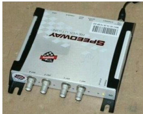
Figure 11 : RFID Reader Speedway R420
