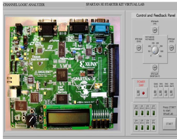
Figure 2.3 - The GUI showing the FPGA development board – Source [2]
