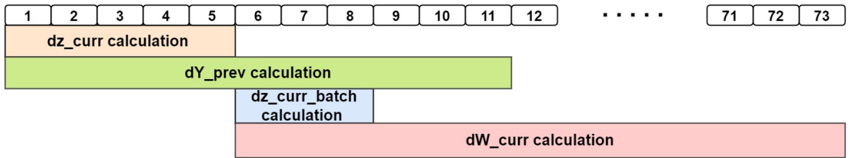
FIGURE 5.21: First Approach - Schedule of the main backpropagation calculations (without db calculation, bias update) in HLS. The number 73 represents the iteration latency (in cycles).
