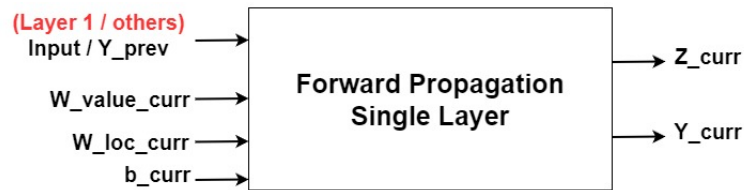
FIGURE 5.2: Single-layer forward propagation block inputs and outputs.
