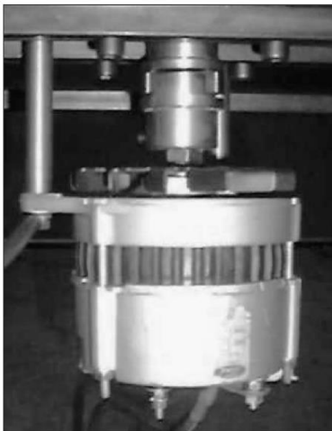
Figure 49. The modified car-alternator under the structure.(Menet, 2004)
