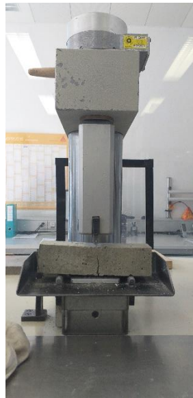
Figure 10: Measurement of flexural strength.
