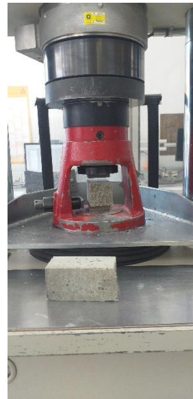
Figure 11: Measurement of compressive strength.
