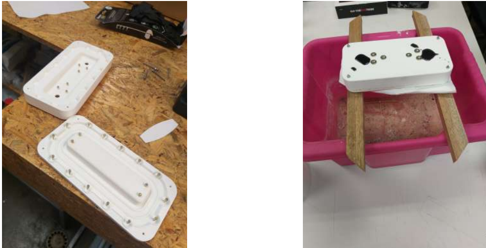
Figure 5.16: The 3D-printed mold for the case on the left, and the mold filled with resin on the right
