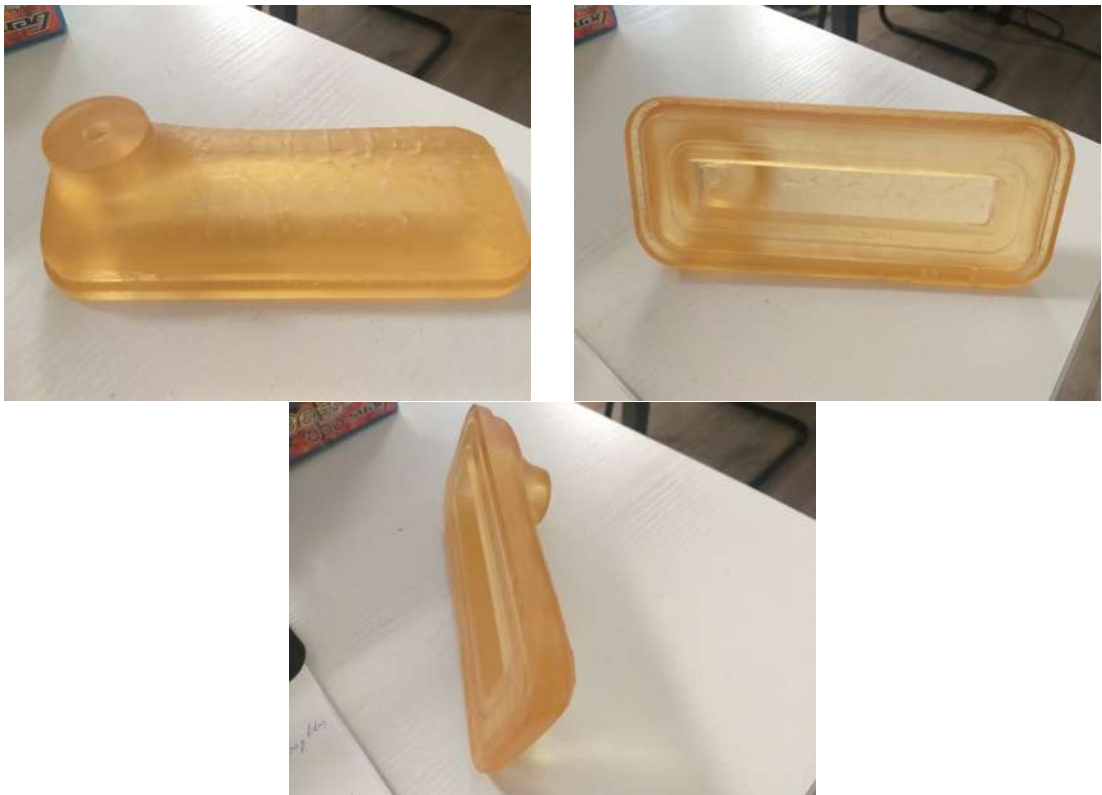
Figure 5.19: Waterproof case just after the Curing Machine
