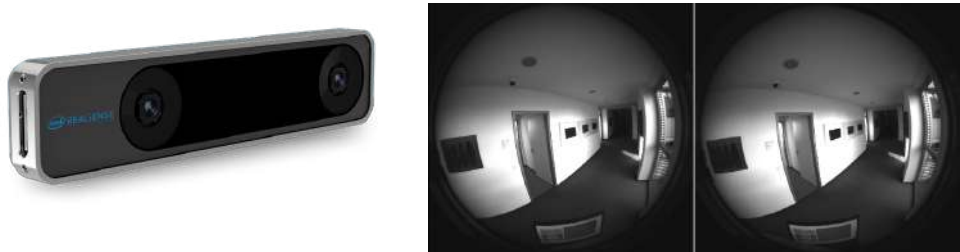
Figure 4.4: T265 tracking camera on the left (source: Intel RealSense) and a frame of the T265 on the right (source: ROS)
