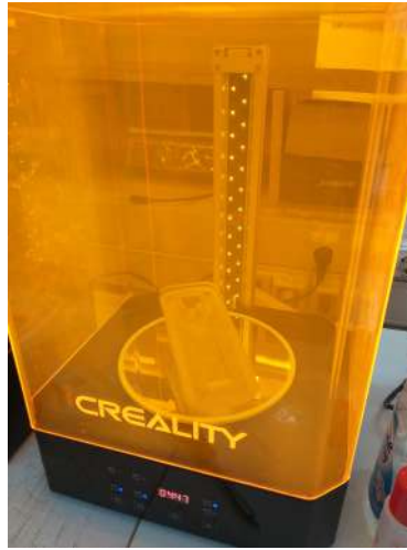
Figure 5.18: Waterproof case inside UV Curing Machine
