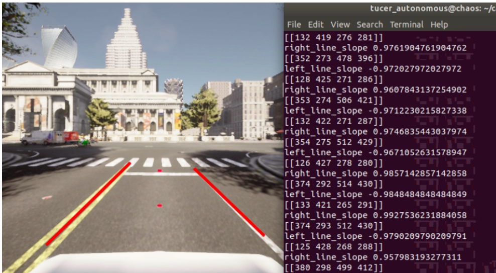
Figure 4.25: Lane Detection with Algorithm Output
