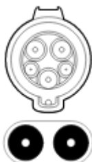
Εικόνα 6-5 Το CCS Combo 1 ( https://www.arrow.com/en/research-and-events/articles/regulations-and-certification-for-electric-vehicles )
