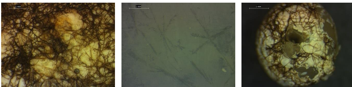
Figure S 11: Stereoscopic images of samples after 300 days in the marine environment (2x magnification): LDPE strip (top left), HDPE strip (top middle), PP strip scope (top right), PS strip (bottom left), PET strip (bottom middle), virgin LDPE pellet (bottom right)
