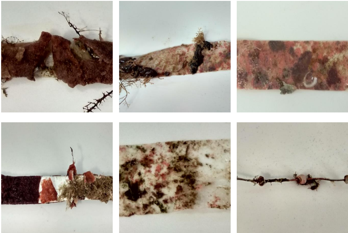
Figure S 10: LDPE strip after 300 days (top left), HDPE strip after 242 days (top middle), PP strip after 300 days (top right), PS strip after 300 days (bottom left), PET strip after 300 days (bottom middle), virgin LDPE pellets after 300 days (bottom right).
