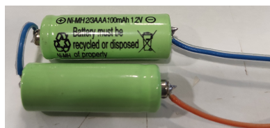
FIGURE 2.10: NiMh 2.4V 100mAh Batteries [12].
