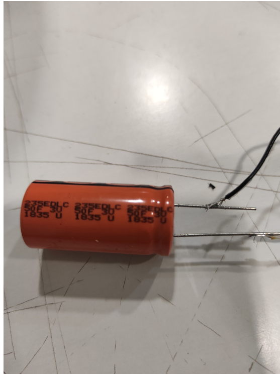
FIGURE 2.6: 3V 50F Capacitor.
