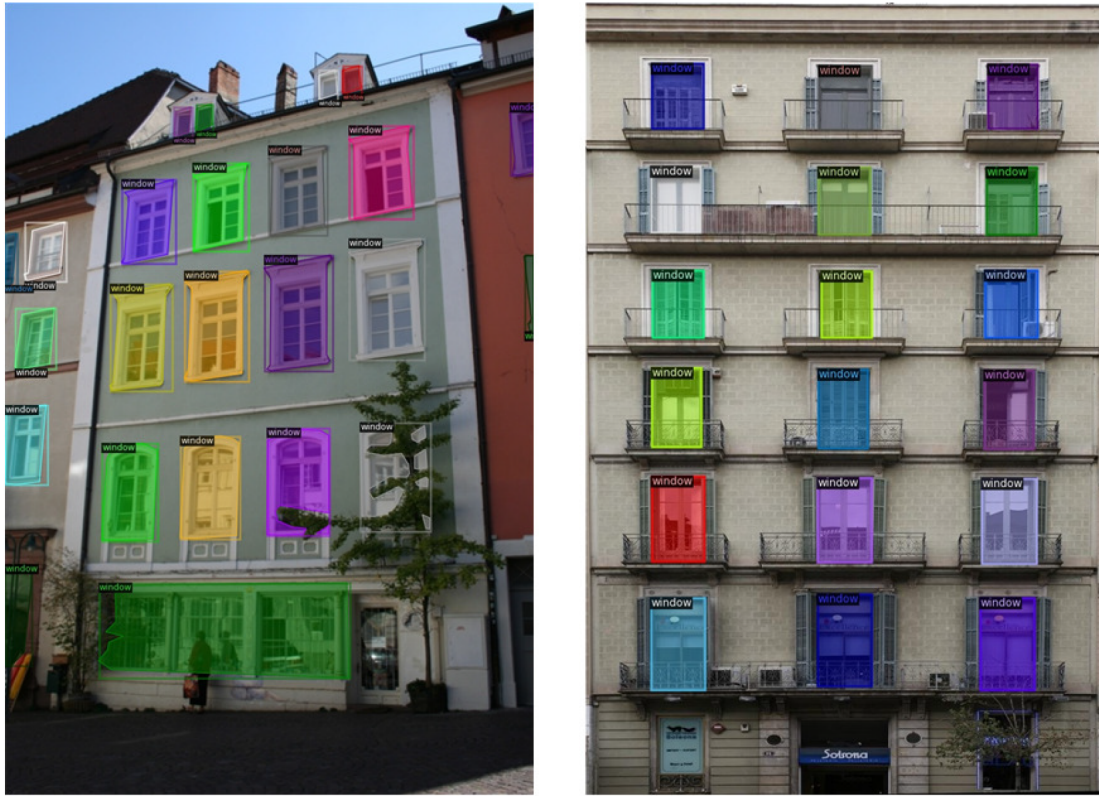
FIGURE 4.10: Window detection using CNN
