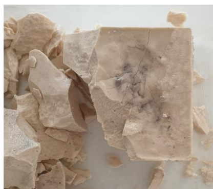
Figure 9. Photo showing the structural deterioration of the MW/MK 0.3 AAM after subjection to 15 freeze–thaw cycles.
