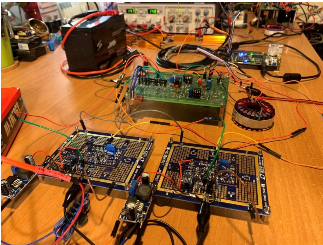
Fig. 24. The experimental prototype of the MPPT and power regulation unit (side view).
