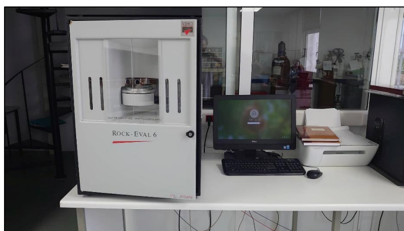
Figure 37. Rock Eval 6 in the lab
