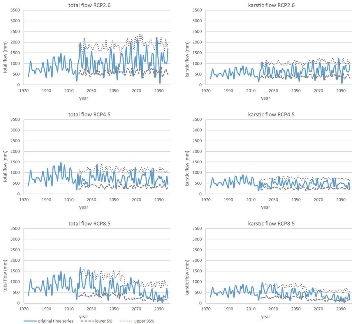
Figure 2.8. Historical data (reference period 1974-2018) and simulations (for the time period 2019 to 2098) of total flow at the Koiliaris basin exit (left) and the respective karstic flow (right). Three different climate change scenarios are used: (top row) RCP2.6, (middle row) RCP4.5 and (bottom row) RCP8.5. The original time series (based on historical data and climate scenario rainfall forecasts) is shown by the blue solid line. The 90% confidence intervals for flow based on the simulated realizations are shown by the dashed (5% percentile) and dotted (95% percentile) lines.
