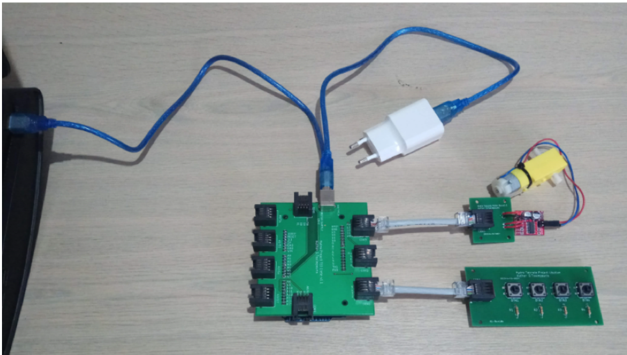
Figure 6. Sample Hydra configuration for DC motor control.
