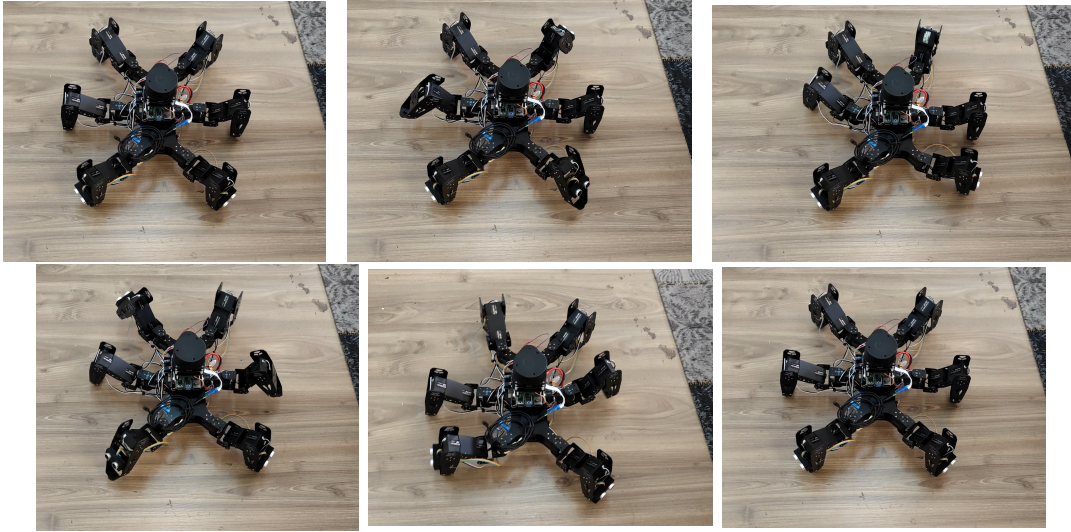
FIGURE 4.24: From top left to right the steps of the tripod gait
