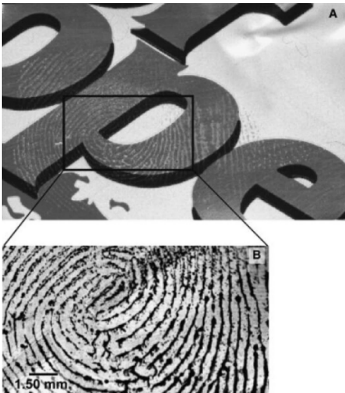
Figure 2.20: Cut and flattened Dr. Pepper's soda can with fingerprint deposit. (A) Soda can imaged by a document scanner. (B) Infrared image of the outlined area obtained by plotting the band intensity at 9842 nm (1016 cm -1 ).
