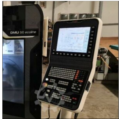
(a) Numerical Control (NC) unit
