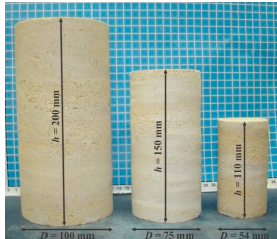
Fig. 1. A series of cylindrical specimens with different diameters for banded Alfas porous stone.
