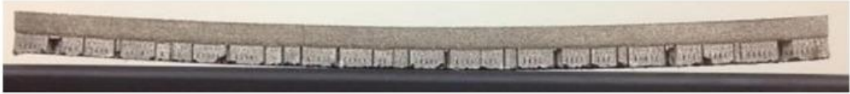
Figure 10. Warpage (Image courtesy of the Centre for Additive Manufacturing and Logistics at North Carolina State University). Taken from [59].
