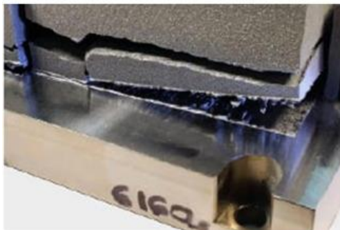
Figure 9. (a) Due to residual stress build-up, a titanium part is removed from the powder bed's build plate. (b) Cracks during the powder-bed process. Taken from [59].
