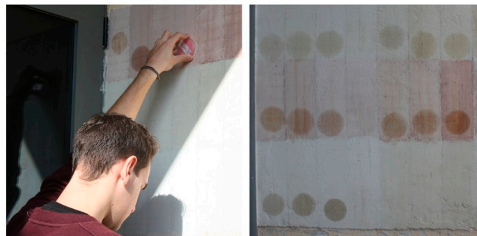
Figure 7. Sponge test (absorption test).
