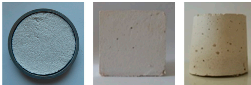
Figure 2. Type of specimens for the laboratory analyses—biscuit, cube, cylindrical specimen.
