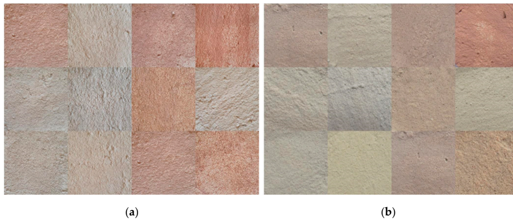
Figure 15. Lime colours on lime plaster: (a) limewater (1:6); (b) limemilk (1:3).
