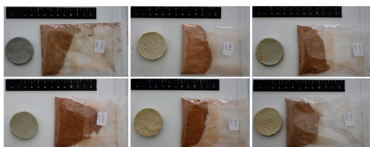
Figure 8. Colour change after heat treatment for samples GLK12, GS7, GA3 (upper, left to right), GK8, GB9, GB6 (down, left to right).
