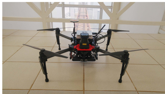
Figure 3. The DJI Matrice 100 quadcopter equipped with the Manifold unit and the Light Detection and Ranging (LiDAR) sensor.
