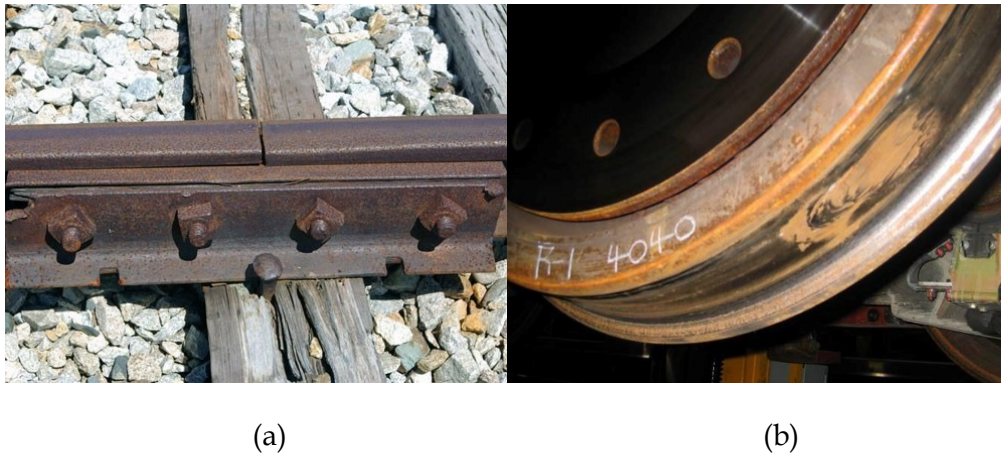
Figure 2.2 (a) Problematic rail joint, (b) wheel flat.
