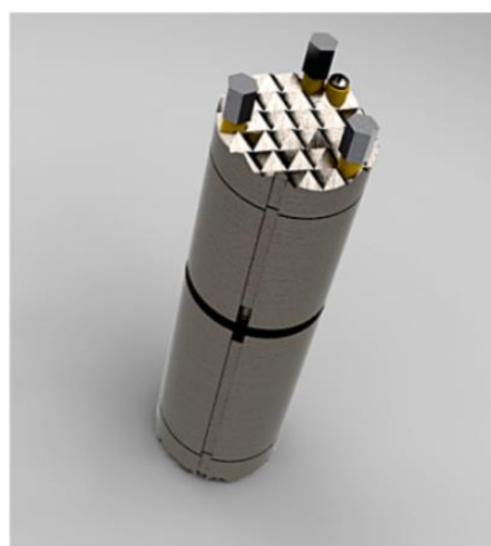
Figure 39 Dual-path ultrasonic cell. Source: (Lin & Trusler, 2012)
