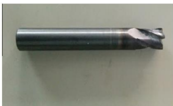
Σχήμα 4.5 Τσιμεντοειδές καρβίδιο (K10) (Πηγή: An experimental investigation on the process parameters influencing machining forces during milling of carbon and glass fiber laminates, N. Rajesh Mathivanan, B.S. Mahesh, H. Anup Shetty, 2016)
