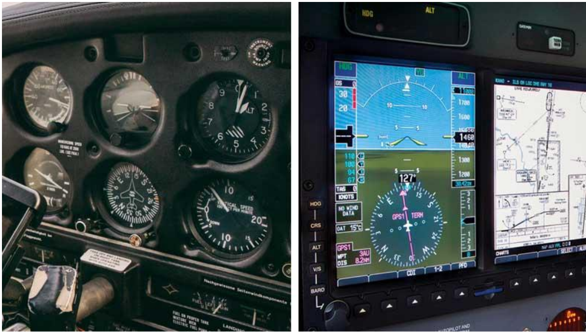
Figure 3.3: Round instruments (Left) vs Glass cockpit (Right) [source: Mid-Continent Instruments and Avionics]
