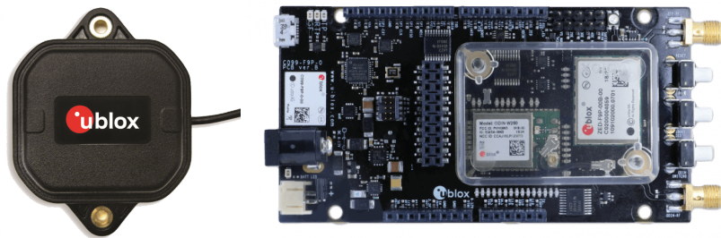
Figure 4.14: (Left) Ublox ANN-MB dual-band GNSS antenna (Right) Ublox C099-F9P application board
