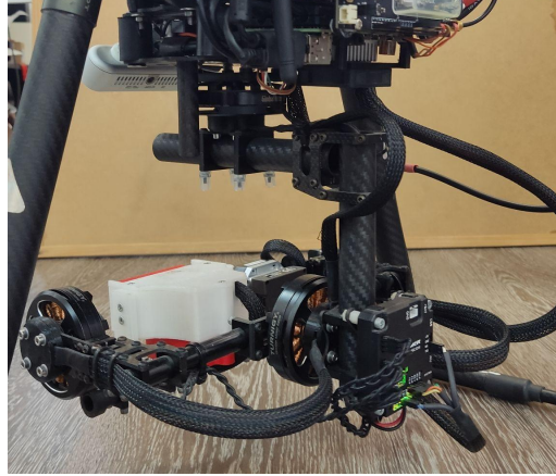
Figure 4.22: The gimbal frame of the geolocation apparatus
