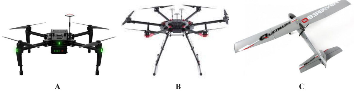
Figure 4.2: Possible UAV configurations, (Left) Option A - Quadcopter [source: DJI Technology Inc], (Middle) Option B - Hexacopter [source: DJI Technology Inc], (Right) Option C - Fixed-wing light aircraft [source: Hobbyking]
