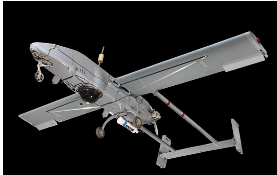
Figure 1.6 (Left) RQ-2A, reconnaissance UAV, source: Smithsonian
