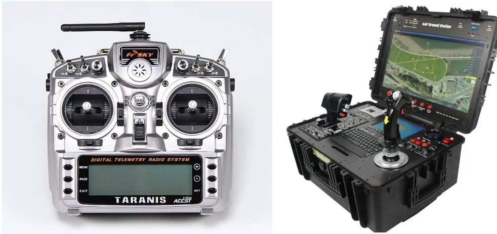
Figure 3.2: (Left) FrSky Taranis X9D handheld radio control unit [source: FrSky], (Right) UAV portable ground station [source: Unmannedrc]
