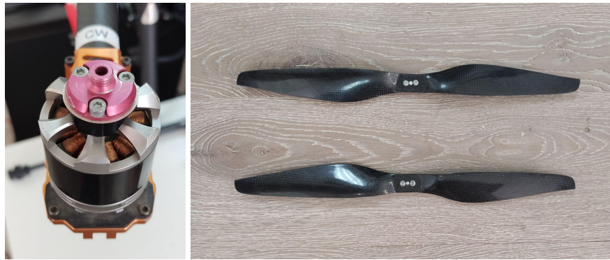
Figure 4.5: (Left) T-Motor MT3520 with a quick release propeller mount. (Right) A pair of CW and CCW carbon fiber propellers.
