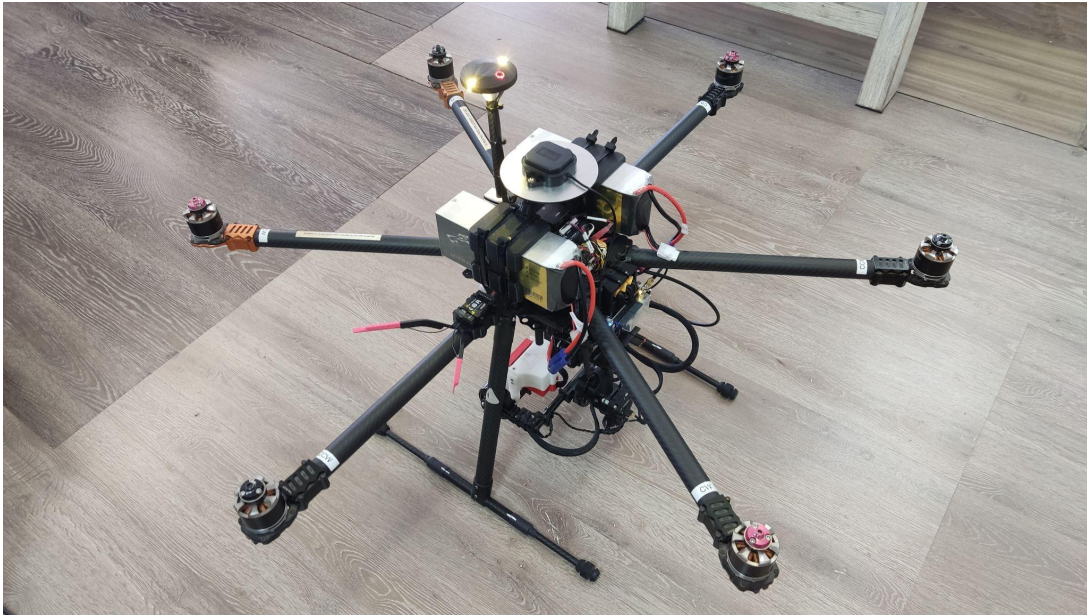
Figure 4.3: The selected hexacopter UAV which will act as the host platform, designed and developed at SenseLab, Technical University of Crete.
