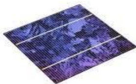
Poly-Crystalline Solar Cell
