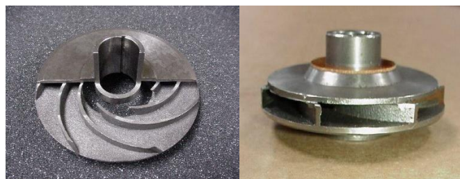
Figure 3. 13 showing sectional view of two impellers and diffusers
