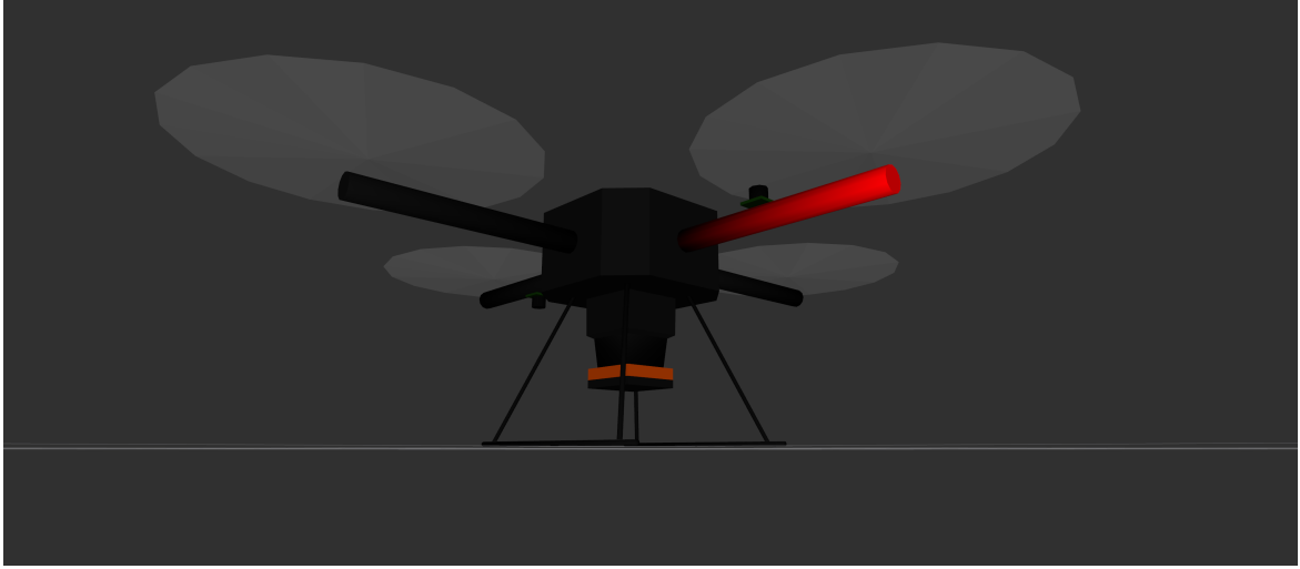
Figure 4.6: A LIDAR sensor is used to provide horizontal obstacle avoidance in a two-dimensional plane.
