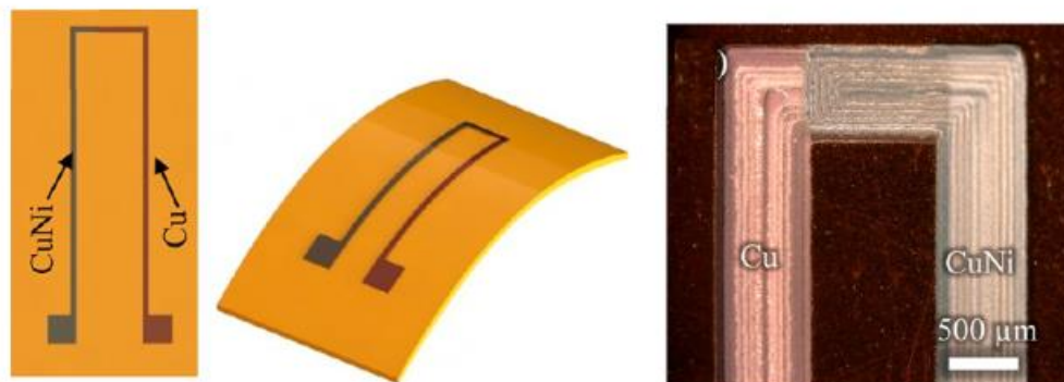
Figure 4.18. AJP flexible temperature sensors deposited on Kapton [183].
