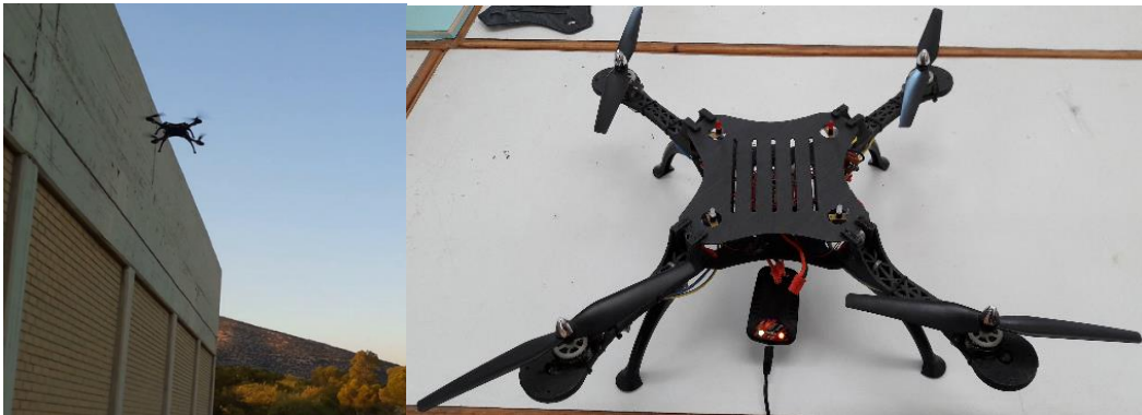
Figure 2.10. 3D printed drone via FDM with carbon fiber filament for defence applications at the Lab of Mechanics of the Hellenic Army Academy.
