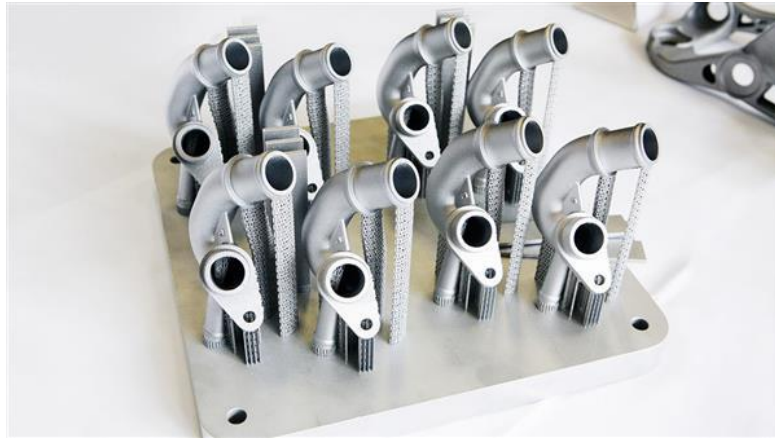
Figure 3.18. Metal 3D printed water connectors for AUDI W12 engine.
