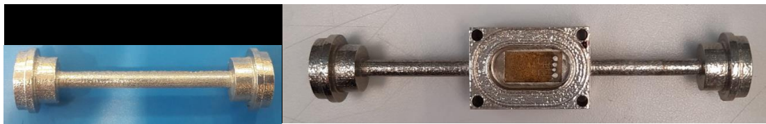
Figure 5.4. The 3D-printed pipe (ID=2mm, OD=3mm) with fluidic connectors (VCR) ( left ) and the 3D-printed pipe with 3D-printed casing, electrical and fluidic connectors ( right ).
