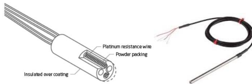
Figure 5.10. Schematic of a coiled RTD configuration.
