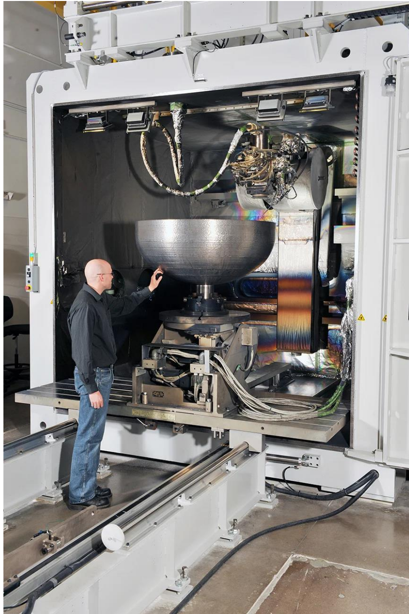
Figure 3.16. An LM worker (for scale) next to their EBM printer and satellite tank dome at the LM space hardware manufacturing facility in Colorado, US.
