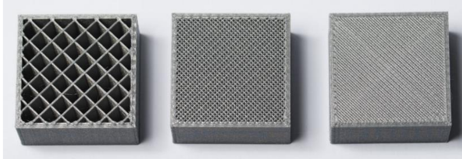
Figure 2.3. Infill percentage of different ranges [35].
