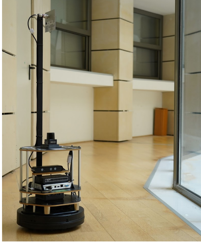
Figure 1.3: Kobuki TurtleBot 2 mobile robotic platform, equipped with a monostatic RFID reader.
