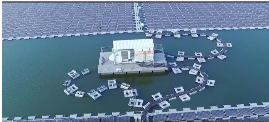
Figure 5: Cabling Routing in Huainan FPV Plant, Eastern China.
