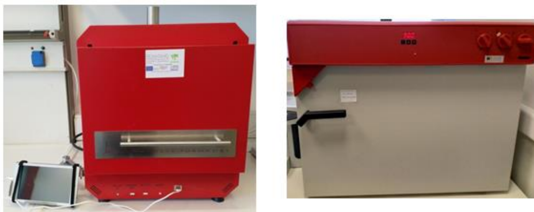
Image 2.2. The furnaces used for the aging and calcination of as-prepared materials (Termansys–left, Binder–right).
