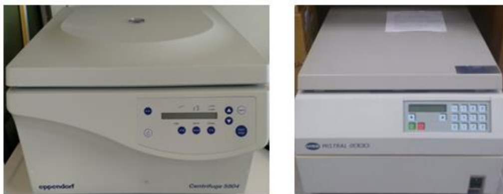
Image 2.3. The centrifuges used for the recovery of the solid products and the washing of the obtained materials with double deionized water and ethanol (Eppendorf centrifuge 5804–left, MSE Mistral 2000–right).
